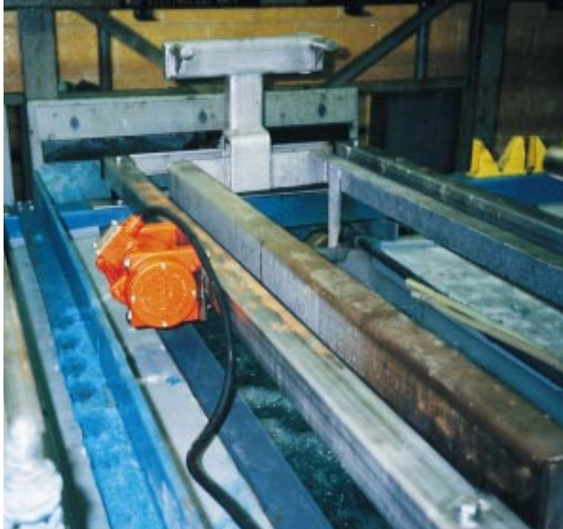
Model 2P-100CE mounted to electroless copper tanks for catalytic activation.
